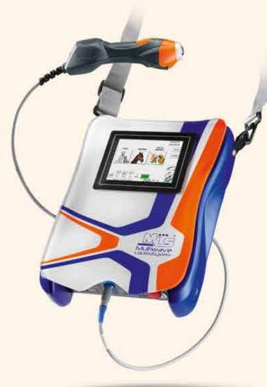
Thanks to the interchangeable head of the handpiece, the standard lens (Target Area of 2 cm diameter) may be quickly and easily removed and replaced with highly efficient guide lights which are able to direct the laser's rays towards much smaller spots to carry out specific treatments for oral conditions and for laser acupuncture.
